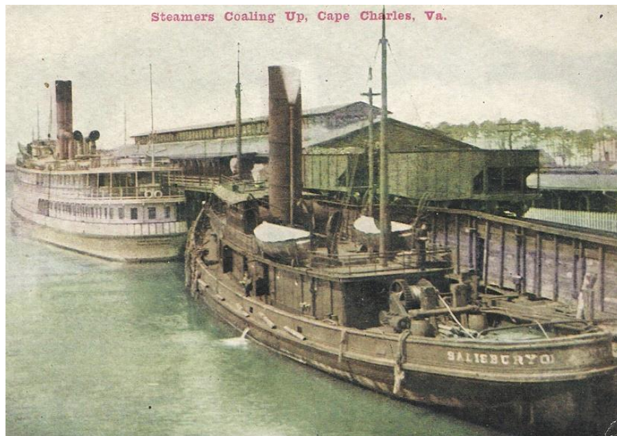
Figure 43 - A NYP&N Railroad steamboat and tug "Salisbury 01" receiving coal in their bunkers for firing the boilers.
